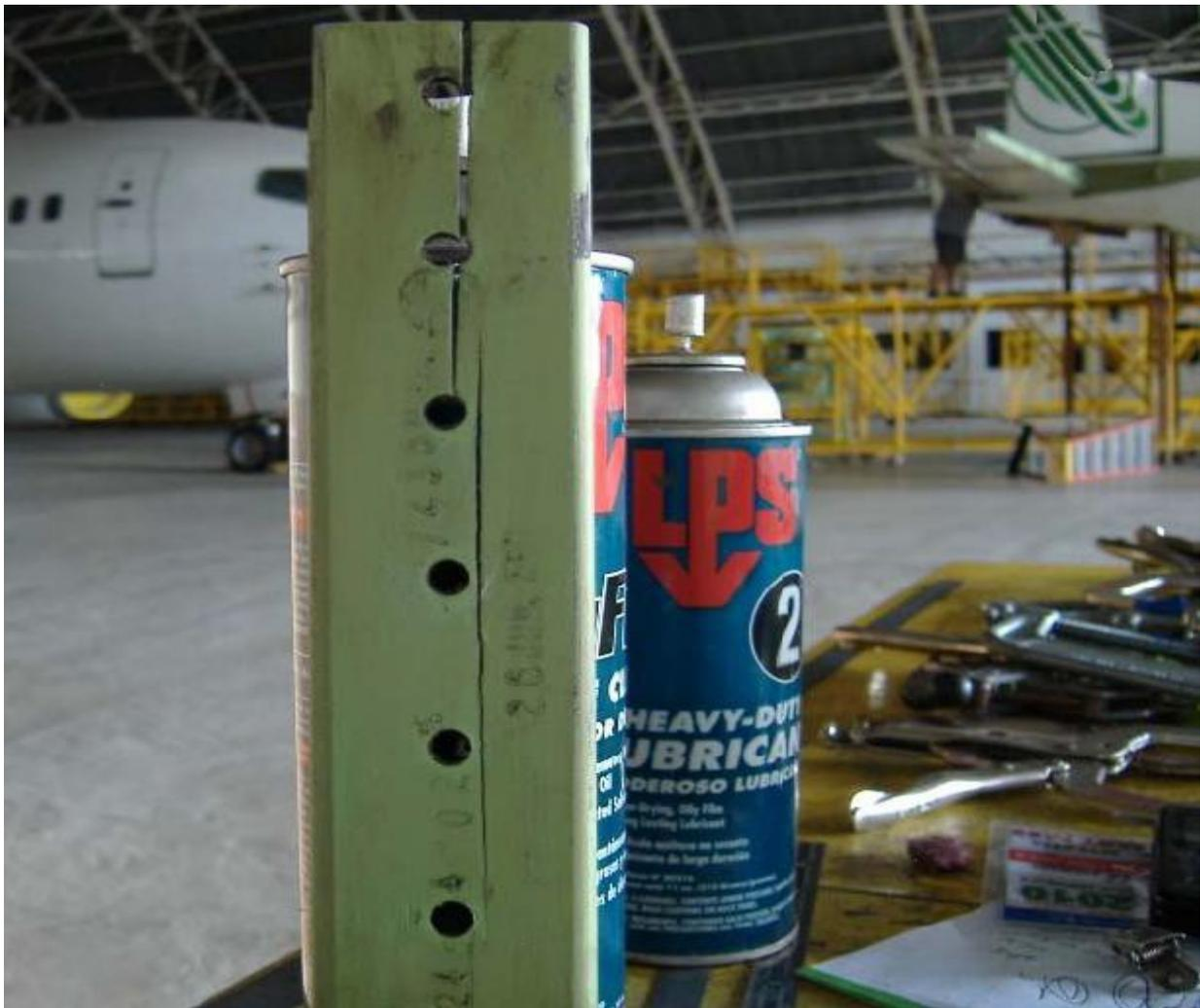
**CASA C212CC, Cracked Horizontal Stabilizer Attach Fittings, ATA 5551**
